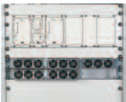
Fig. 4: Modular power supplies fitted into card frame. Power supplies can be sized so that any single module failure will not affect the system. Hot-swappable for quick field service.
